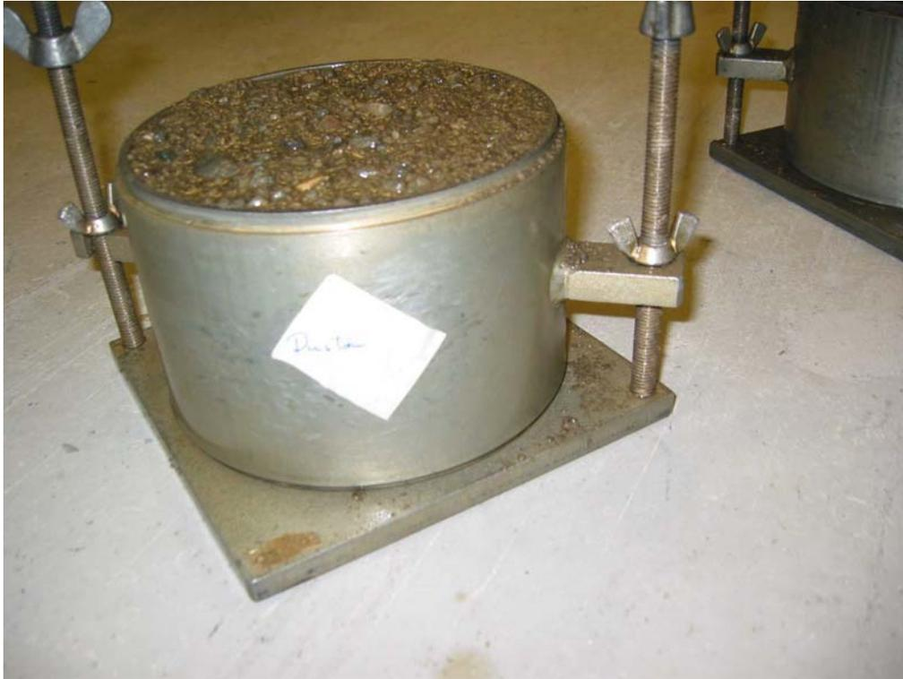
**Figure 1 Sample with DUSTEX after compaction**
